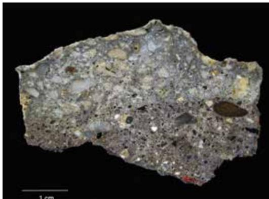
Scratched plaster: sample / transversal view under angled light / daylight. The white, greyish crystal clasts are travertine. The gray aggregates presumably show Osnabrück shell limestone with enclosed iron oxide-containing anchorite components, which are typical of yellowish surface weathering.
