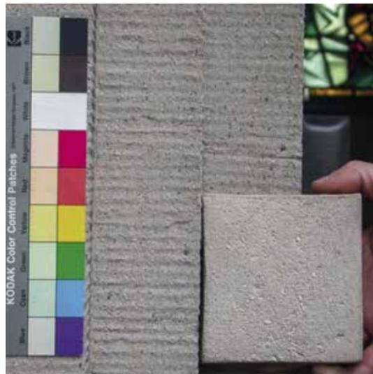
Repair mortar we assembled in comparison with the construction concrete block at the stucco border of the entrance area.
