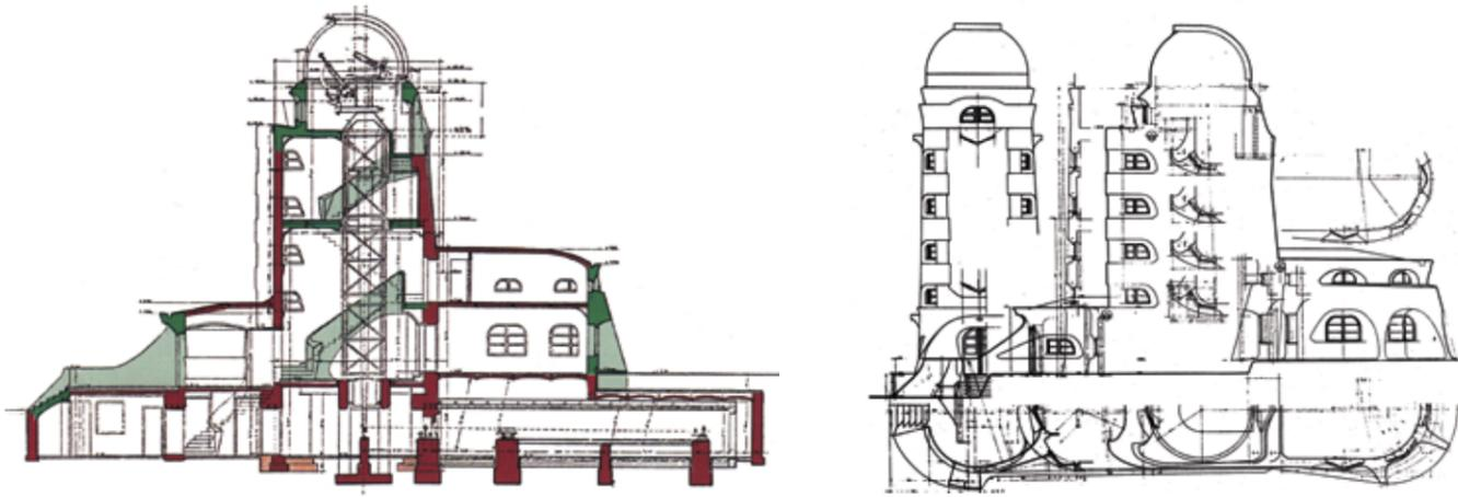
(left) Potsdam, Telegrafenberg, Einstein Tower 1920-1922, Architect Erich Mendelsohn. Mapping of the mixed construction. Red: brickwork, green: reinforced concrete. Graphics, Huse 2000, p.93, Gerhard Pichler.
