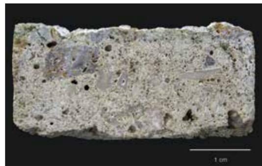
Peine, Lessing Lodge, east facade, stone plaster / sample: Both pictures show large paneled gypsum crystals.
